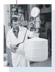
We have the capability to grow high-quality large size alkali halide crystals for scintillation applications.
