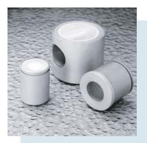
A well-type receptacle in NaI(TI) detector provide maximum absorption of radiation from a sample by approximating 3  $\pi$  geometry. Both open window detector and integral assemblies are available. Typical housing wall thickness is 1/32". We can design the special well sizes detectors upon customer request.
