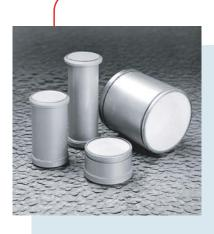
All crystals are hermetically sealed in aluminum housing. Copper or stainless steel housings are available for special (low background) applications. UV transmitting glass is used for the optical window. Standard housing wall thickness is 1/32". Special low-mass entrance windows are also available.
